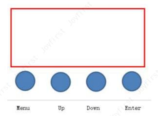
MENU DOWN UP ENTER To select the programming functions To go backward in the selected functions To go forward in the selected functions To confirm the selected functions
