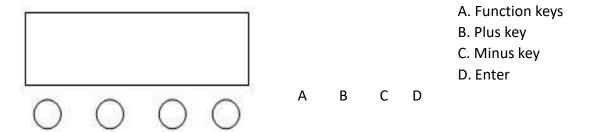
Operation instructions: Press function key A to cycle through different functions, and press B or C key to modify its parameter values. Press D key to confirm.
